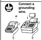
■ Ensure that the equipment is properly grounded. Extension cables should also be grounded. Fire or electric shock can occur on improperly grounded equipment.
